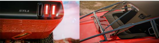
To ensure no landscape on earth can impede the STL1's stampede, the team have upgraded the suspension with high performance billet coil-over shocks, tubular upper and lower full A-frame style control arms at the front, and completely redesigned upper and lower tubular heavy duty rear control arms. To help it stop on a dime, the front features drilled and slotted 11" brake disc rotors paired with heavy duty aluminium callipers, with 10.5" inboard-mounted units at the rear, à la the Alfa Romeo SZ.
